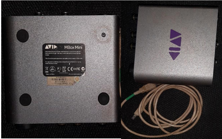
Audio Interface - AVID Mbox Mini 3rd Generation Ultra-compact 2x2
